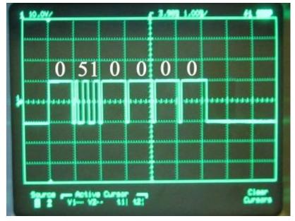
This is a closeup of the instruction byte 2. The "S" on either end represents the start and stop bits respectively. The start bit is always positive and the stop bit is always negative. The bit sequence is Start, 0, 1, 2, 3, 4, 5, 6, 7, Stop. The data is output with the least significant bit first, so the byte shown is actually 00110011 in binary or 32+16+2+1 = 51 in decimal.
