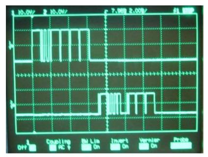
This is a closeup of the instruction bytes. Note that the voltage swing of the instruction waveform is about +/-10V. This is typical of the USB to RS232 converter to which the device is connected. The instruction bytes are 0, 51, 0, 0, 0, 0 indicating the instruction: Device: All, Command: Return version, Data: 0.
